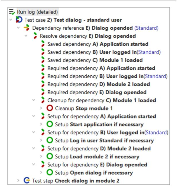
Figure 8.7: Dependency stack A-B-D-E
