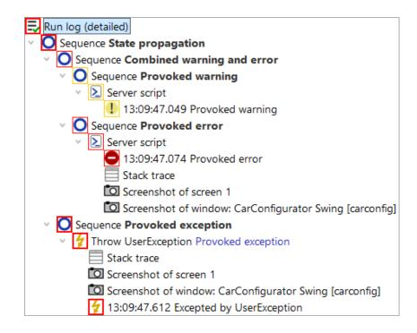
Figure 7.2: Error states in a run log
