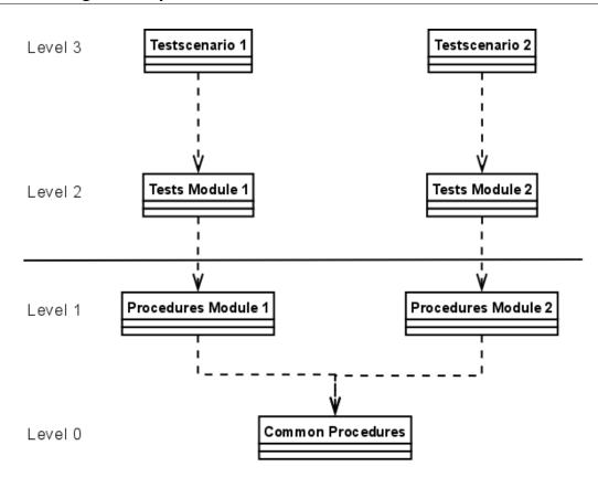
Figure 35.1: Structure of multiple test suites
