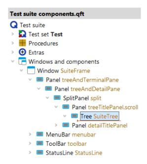
Figure 5.9: Component hierarchy of a Swing SUT
